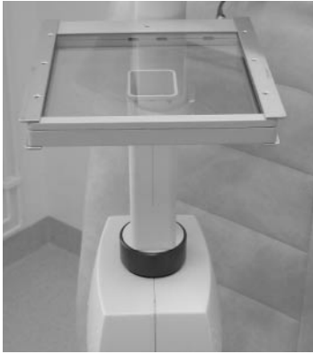
Figure 1. Transmission ionisation chamber for measuring of DAP values in an intraoral unit.
