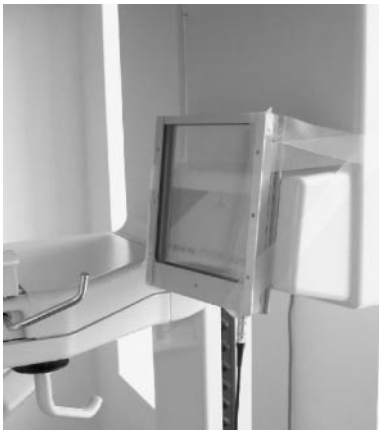
Figure 2. Transmission ionisation chamber for measuring of DAP values in a panoramic unit.
